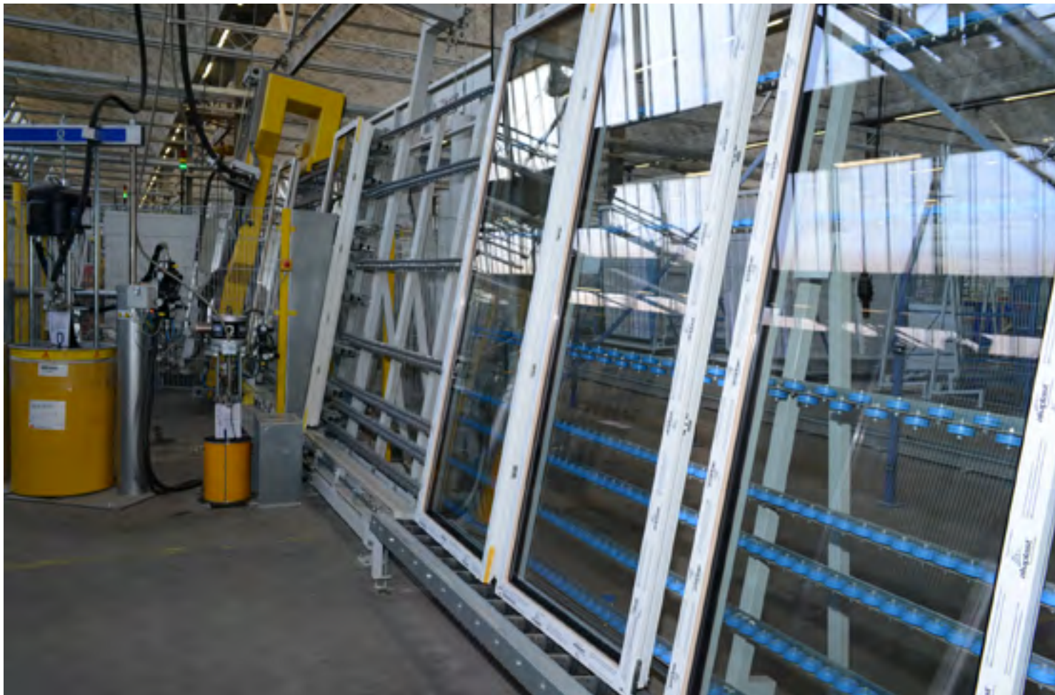
The consistently high quality of our products is largely due to the method of bonding the insulating glass in the sash frame – what we call the 'bonding inside' technology.
