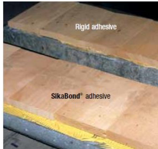
Testing under extreme conditions: 21 mm thick massive beech board, 22 % wood moisture content
