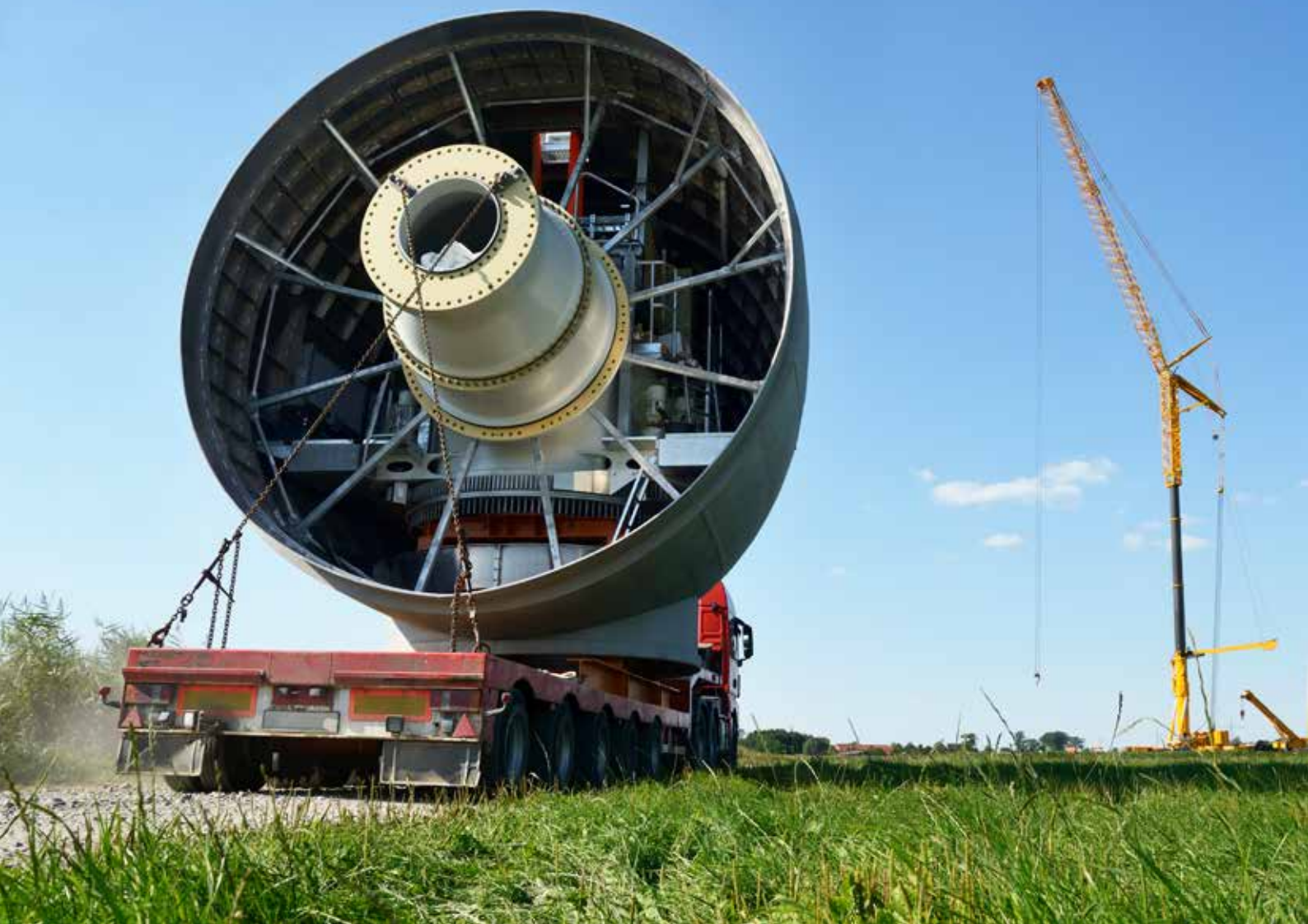
Hub transport to the erection site of the turbine.
