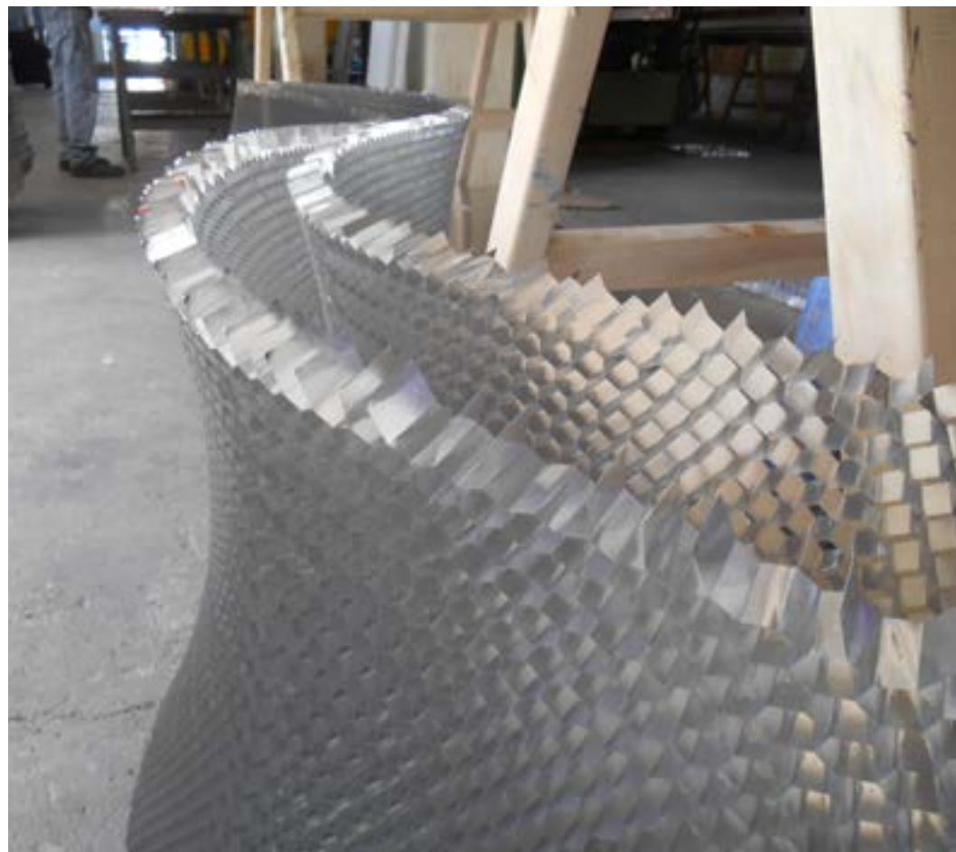
Honeycomb panels can be installed in large dimensions, have excellent rigidity and flatness and reduce the weight of the structure.
